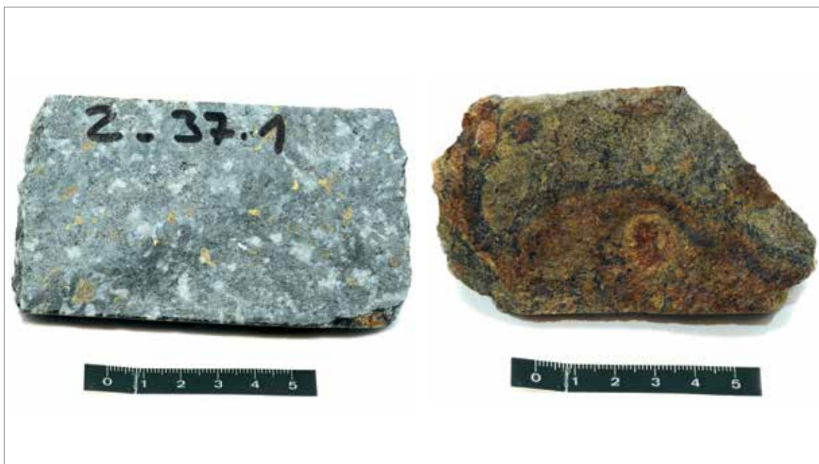
Fig. 4.19: The comparison of a fresh (pristine, left) to an oxidised (right) PGM bearing ore from the Platreef (drill core samples from the Mogalakwena Mine, Anglo Platinum Ltd.).
