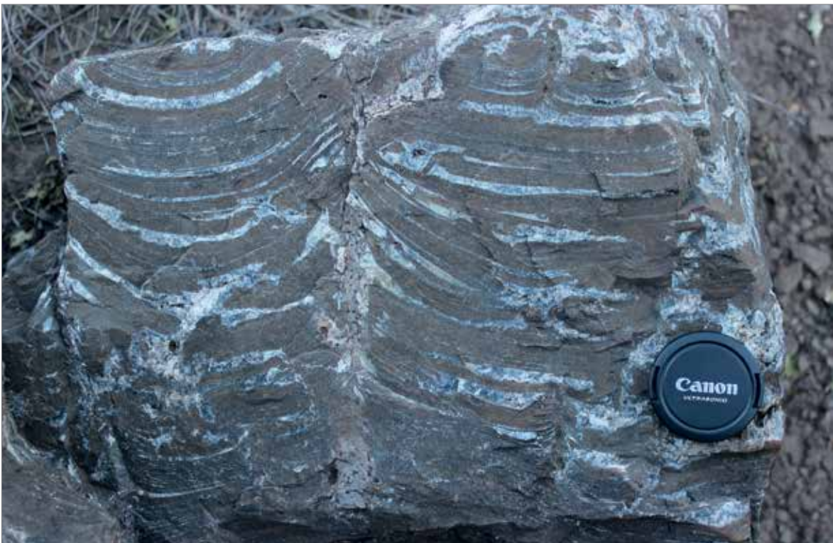
Fig. 2.21: Stromatolite sample from "R7" with layers of fluorite, which has replaced the original calcite (photo: DERA 2014).
