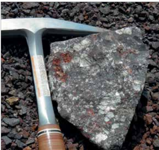
Fig. 2.14: Rock sample from Vergenoeg mine with fluorspar in a magnetitic matrix (photo: DERA 2012).
