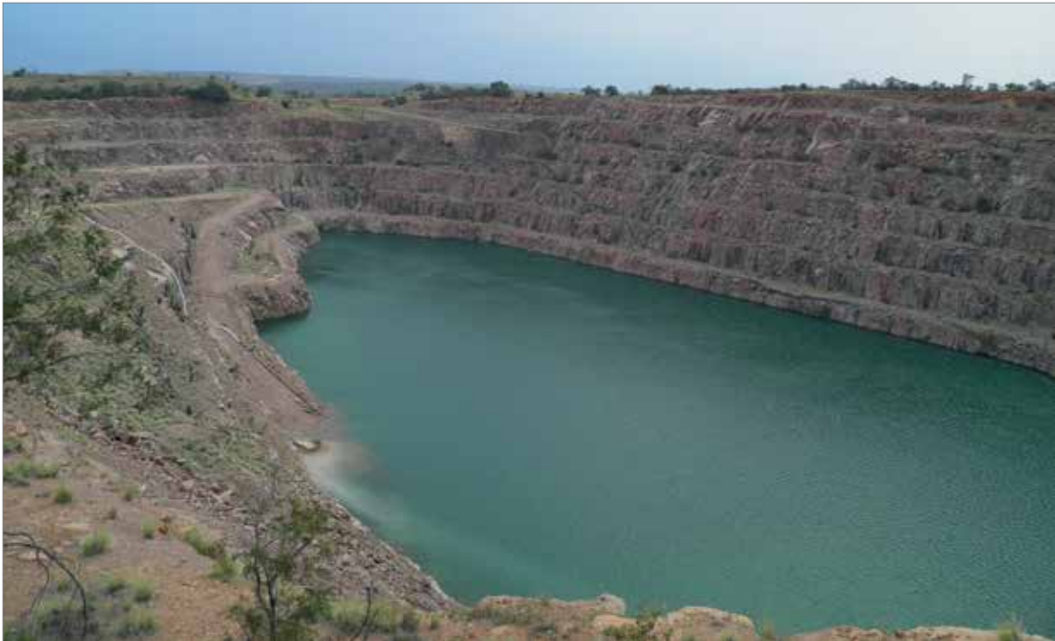
Fig. 2.18: The northern pit (the North Kloof, closed since 1994) of the three open pits from the Buffalo Mine with an N-S extension of about 320 m and a depth of 100 m (photo: DERA 2013).
