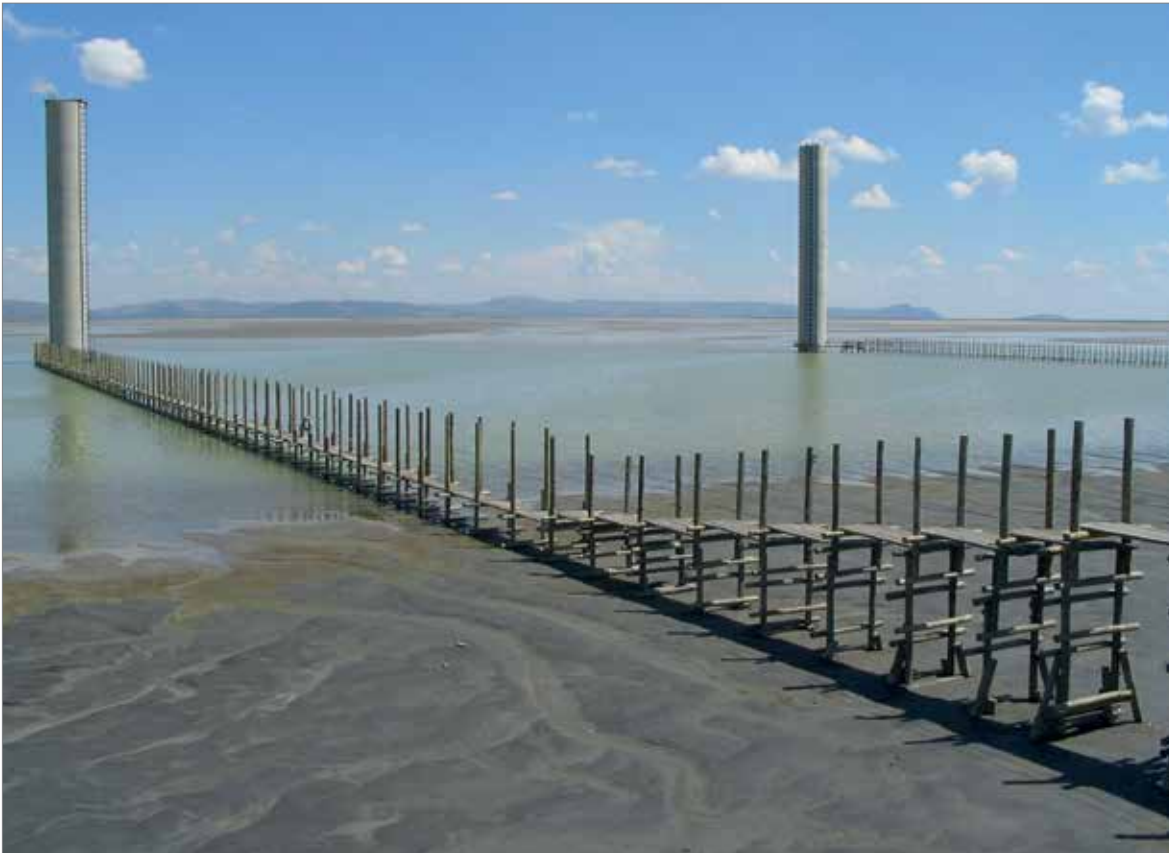
Fig. 5.3: Tailings dump at Impala Platinum Mine (about 220 Mt material containing 0.7 ppm PGE-4E; photo: BGR 2008).
