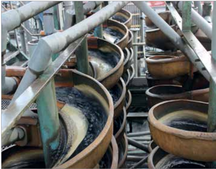
Fig. 5.6: The spiral separation facility (left) at Moolinoi plant (right), in the western Bushveld, for recovering chromite from tailings material (photos: DERA 2014).
