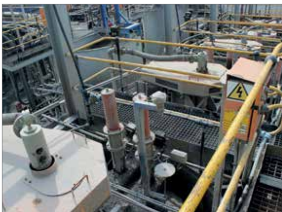
Fig. 5.7: Flotation equipment for producing PGE concentrates at Moolinoi plant (left). PGE bearing sulfide minerals are concentrated within the foam (right) (photos: DERA 2014).
