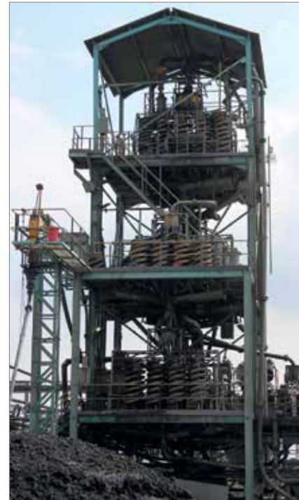
Fig. 5.6: The spiral separation facility (left) at Moolinoi plant (right), in the western Bushveld, for recovering chromite from tailings material (photos: DERA 2014).
