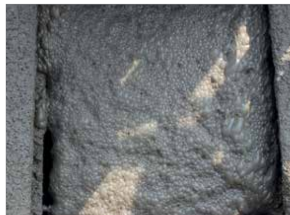
Fig. 5.7: Flotation equipment for producing PGE concentrates at Moolinoi plant (left). PGE bearing sulfide minerals are concentrated within the foam (right) (photos: DERA 2014).
